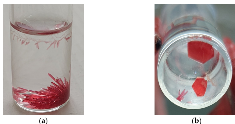
Figure 2. Photos of crystals obtained from the recrystallization of powders of [\text{Ni}_x\text{Zn}_{(1-x)}(\text{bpy})_3](\text{PF}_6)_2 : (a) 10% Ni and 90% Zn (needles); (b) 50% Ni and 50% Zn (needles + plates). Vials shown are 13 mm in diameter.
