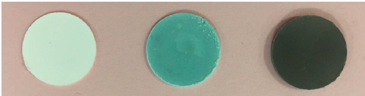
Figure 3. Zeolite samples pressed into pellets: parent zeolite MOR (left), MOR-Cu(NO 3 ) 2 before activation (middle), and MOR-Cu(NO 3 ) 2 after activation (right).
