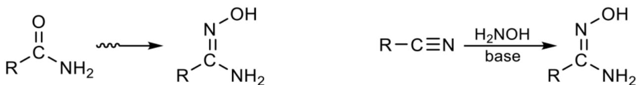
**Figure 1.** The relationship between primary amides and amidoximes (left) and the typical route for the synthesis of amidoximes (right). The term “amidoxime” is frequently used for compounds with the  $-NR_2$  group (R = alkyl, aryl, etc.), but, in this review, the name is confined to molecules possessing the  $-NH_2$  group.
