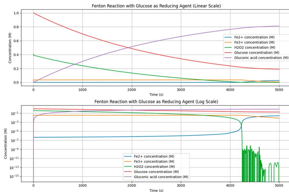
**Figure 9.** Python simulation of Fenton oxidation of D-Glucose.
