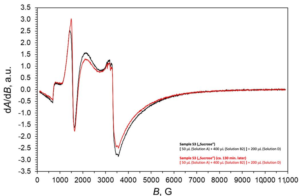
Figure 6. EPR spectra time dependency of Sucrose oxidation.
