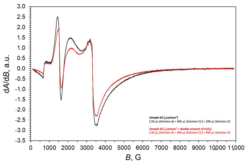
Figure 4. EPR spectra of D-lactose oxidation using different amounts of  $H_2O_2$ .
