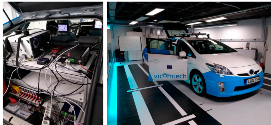
Figure 7. Pictures of our test car, CarLOTA, including a picture of all the equipment installed in the trunk of the car.
