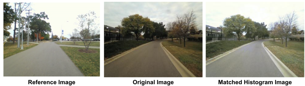
Figure 13. Example of the histogram pre-processing technique used to balance images obtained from the front vehicle camera.
