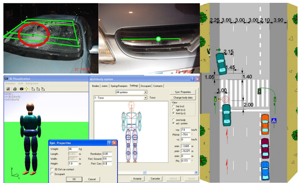
Figure 2. Setting the initial conditions of the reconstruction in PCCrash©, considering the multi-body model of the pedestrian and the impact zone.
