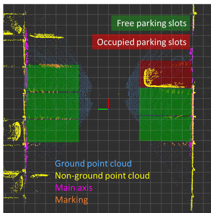
Figure 5. Detected parking slots.
