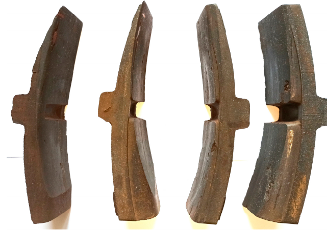
Figure 1. Unusable composite brake pads with wedge-dual wear and significant reduction of their working parts.
