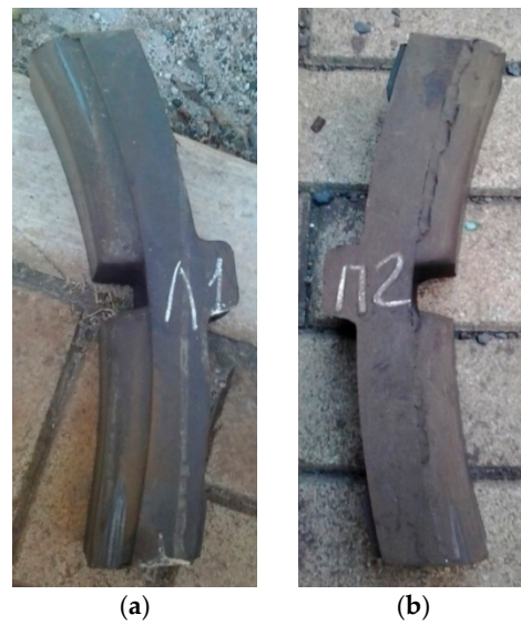
Figure 3. A sample a composite brake pad with uniform wear with regard to the thickness: (a) the first brake pad in the running direction (marked as Π1); (b) the second brake pad in the running direction (marked as Π2).
