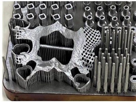
Figure 15. RPD after SLM.
