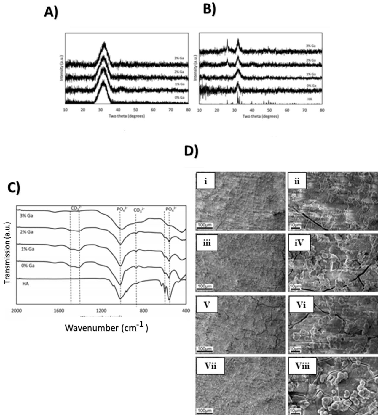
**Figure 2.** (A) XRD spectrum for unreacted BG; (B) XRD spectrum for BG after 7 days in SBF, with hydroxyapatite shown as a reference; (C) FTIR spectra of Ga doped BG following immersion for 7 days in SBF; (D) SEM image of BG after 7 days in SBF. (Adapted from [3]).
