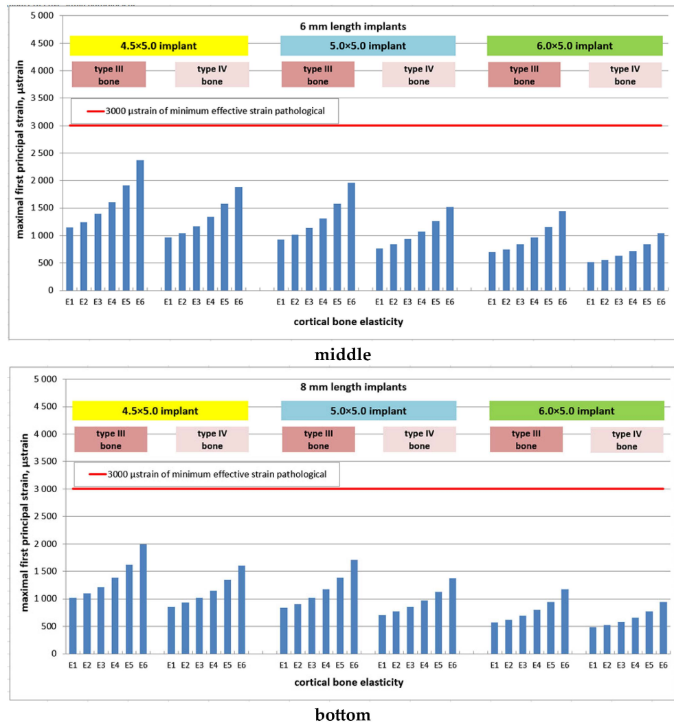
Figure 7. Dependence of maximal first principal strains (MFPSs) in cortical bone on its modulus of elasticity for implants of length 5.0 mm (top), 6.0 mm (middle), 8.0 mm (bottom) placed into bone segments of type III and IV bone and the studied E1–E6 degrees of patient-specific cortical bone elasticity. Red line corresponds to 3000 microstrain of Frost “minimum effective strain pathological” (MESP).
