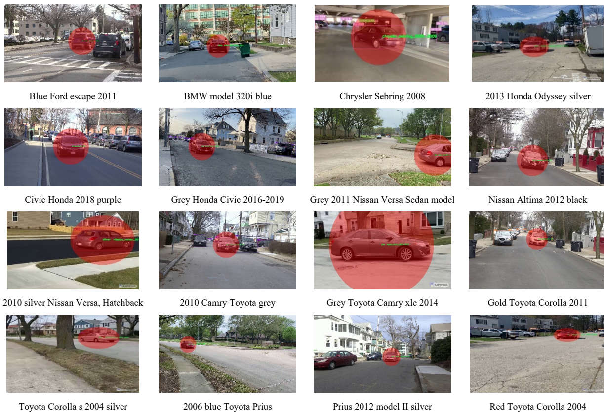
Figure 11. Sample results for vehicle search and localization. The tags below each image represent simplified or preprocessed text-input queries. The red circles are the corresponding localizations based on the input queries. Sample results shown here are based on extracts from the video VRiV testbench dataset, and the localizations match the corresponding ground truth based on query.
