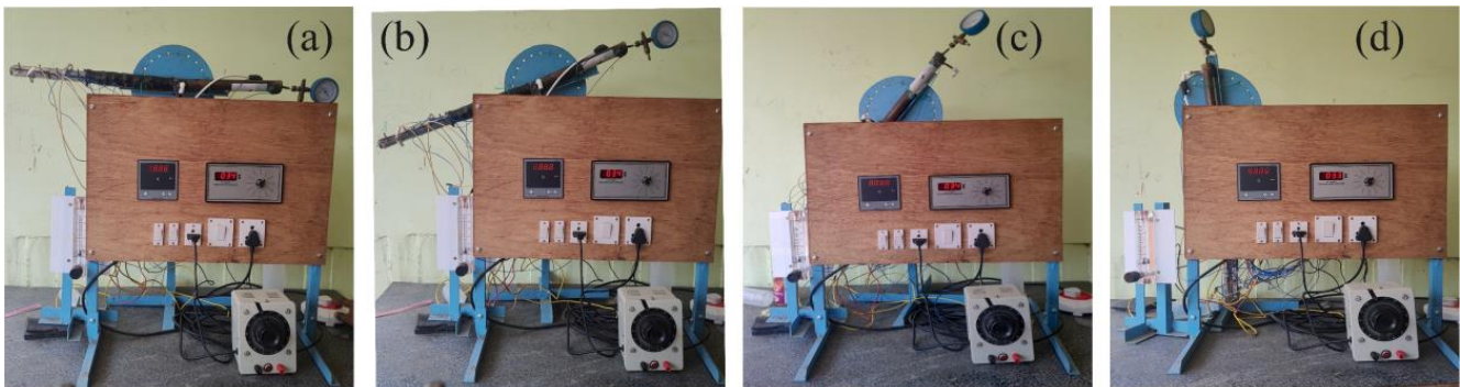
Figure 5. Schematic view of the experimental setup based on angles (a) 0^\circ , (b) 45^\circ , (c) 60^\circ , and (d) 90^\circ .
