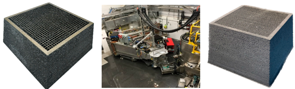
Figure 36. Neutron scattering instrumentation at the Spallation Neutron Source of ORNL (middle), boron carbide MMC 3D collimator (left), and 2D collimator (right).
