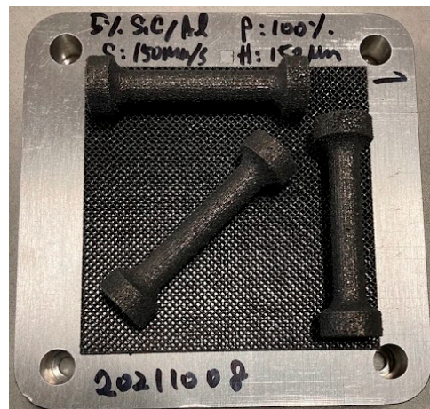
Figure 15. Example of standard dog-bone parts printing.
