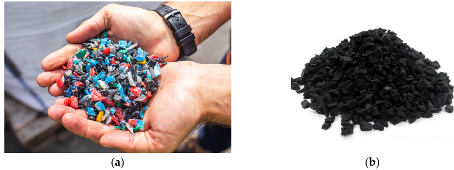
Figure 1. (a) Plastic aggregate and (b) tyre aggregate.
