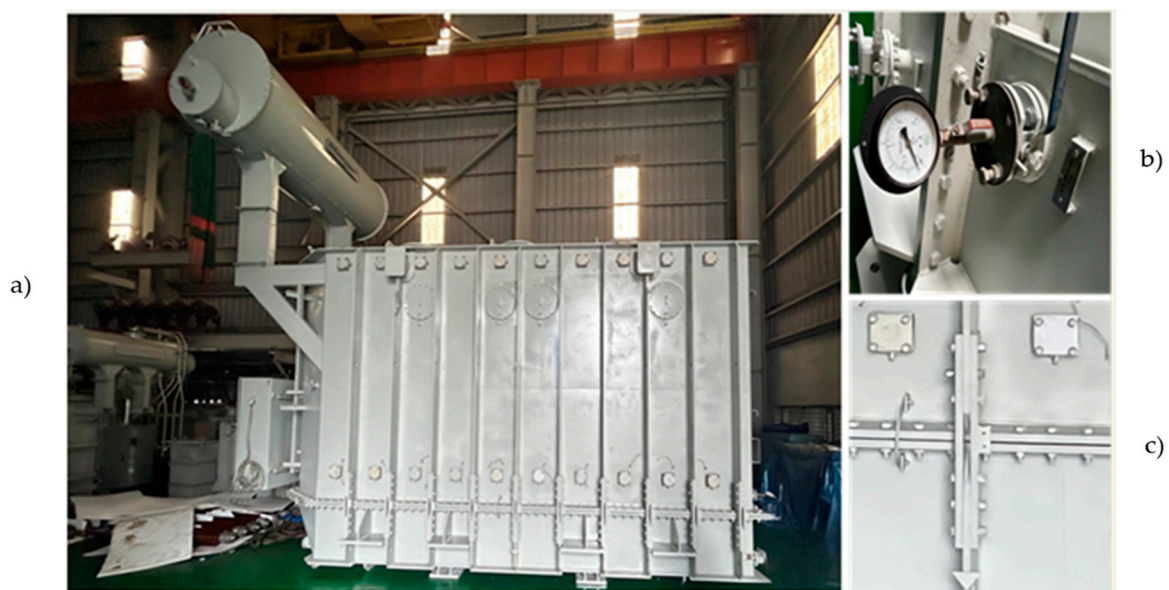
Figure 6. (a) Experimental setup for pressure testing of 120 MVA 132/33 kV power transformer tank. (b) Set up the pressure gauge meter; (c) Supports are installed on both sides of the stiffeners.
