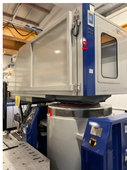
Figure 3. Sinusoidal sweep test device: (1) vibration test device, (2) climatic chamber.
