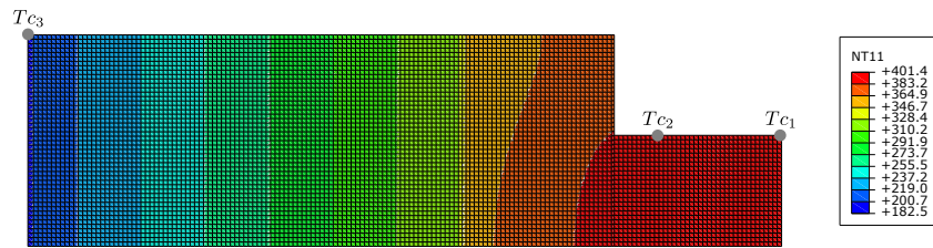
Figure 7. Temperature contourplot in the anvil and the sample at the end of the heating phase ( t = 1100\text{ s} ) for the constant cooling condition.
