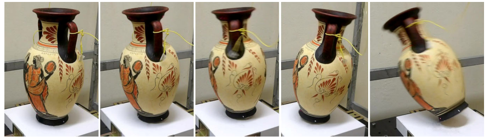
Figure 15. Photographs showing the seismic response of the amphora (small coefficient of friction). Rotation of the amphora about its vertical axis is observed.
