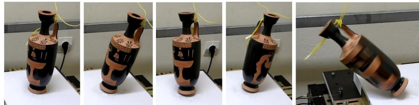
Figure 5. Photographs showing the seismic response of the large lekythos (small coefficient of friction). Rotation of the large lekythos about its vertical axis is observed.
