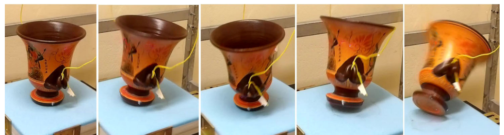
Figure 23. Photographs showing the seismic response of the krater (large coefficient of friction).
