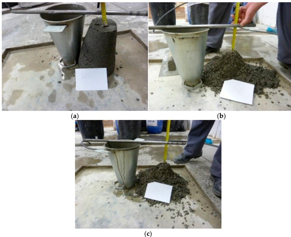
**Figure 7.** Slump test of RmCs: (a) 0 vol% rubber, (b) 10 vol% rubber, and (c) 20 vol% rubber.
