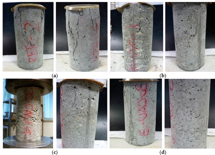
Figure 11. Failure modes of RmC specimens under compressive testing: (a) 0 vol% rubber; (b) 10 vol% rubber; (c) 20 vol% rubber; and (d) 30 vol% rubber.
