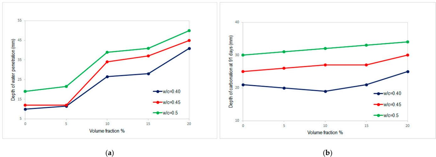
**Figure 1.** Relationship between durability performance and w/c at various volume fraction of crumb rubber: (a) depth of water penetration and (b) depth of carbonation (mm). Data have been adapted from Thomas and Gupta [24].
