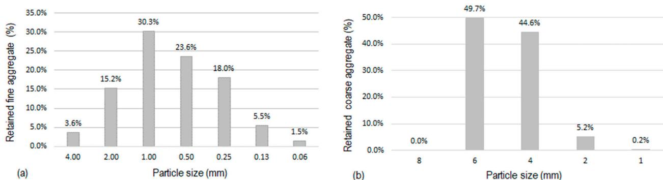
**Figure 2.** Granulometry of the aggregates: (a) fine aggregate (0/4-R-S) and (b) coarse aggregate (0/6-T-S).
