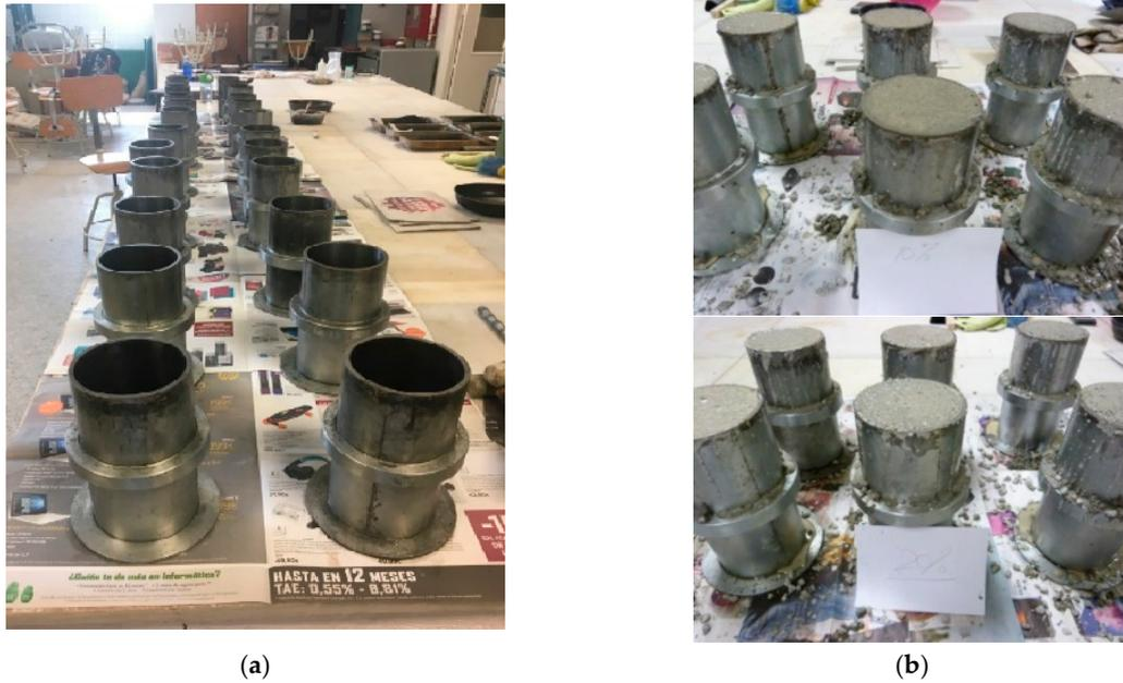
**Figure 6.** Manufacture of test specimens: (a) molds of the test pieces and (b) pouring of fresh micro-concretes.
