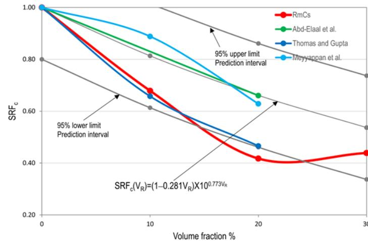
Figure 10. Strength reduction factor of compressive strength in RmCs [24,79–81].
