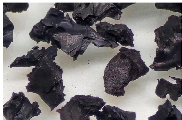
**Figure 4.** Surface finish of the recycled rubber particles.
