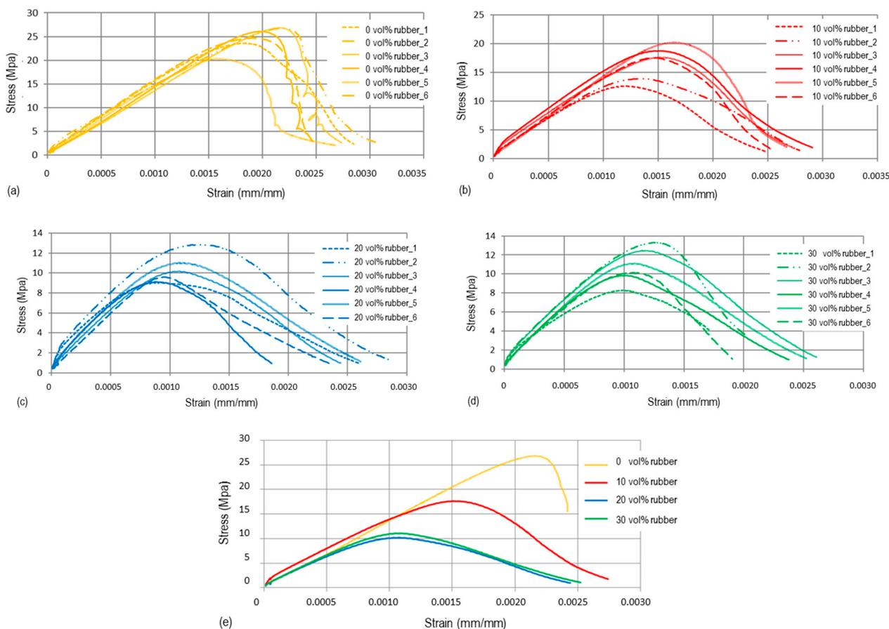
**Figure 9.** Compressive stress–strain curves of RmCs: (a) 0 vol% rubber; (b) 10 vol% rubber; (c) 20 vol% rubber; (d) 30 vol% rubber; (e) average results.
