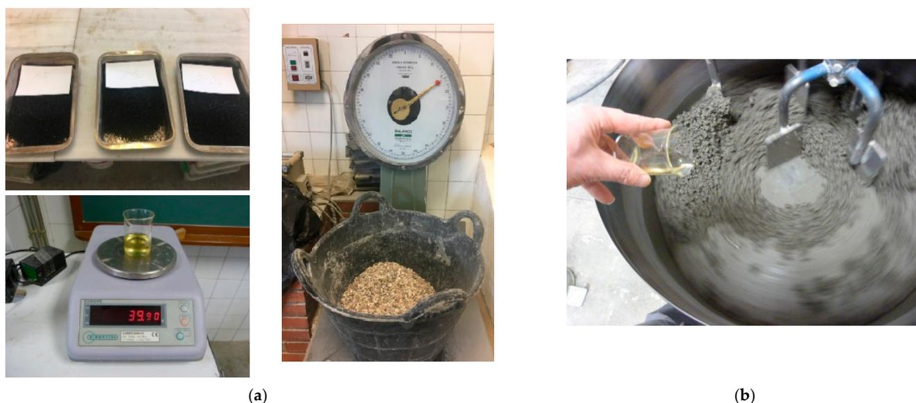
Figure 5. Manufacture of test specimens: (a) weighing and (b) mixing of the materials.
