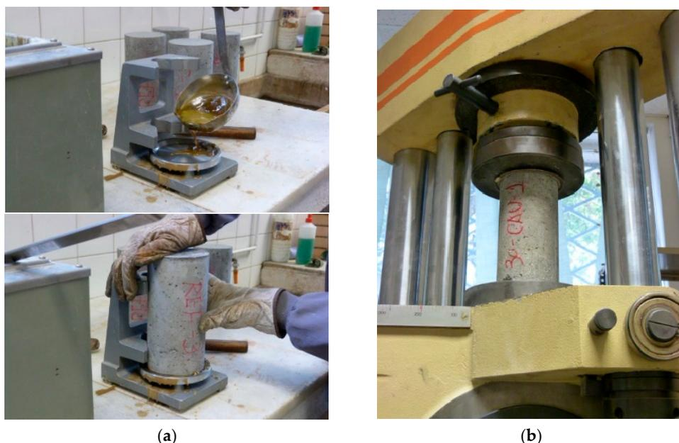
**Figure 8.** Compressive strength test: (a) specimens capping and (b) test.
