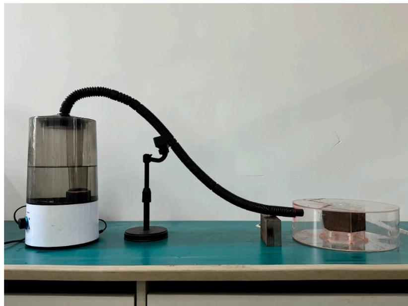
Figure 3. Fog chamber water collection detection device.
