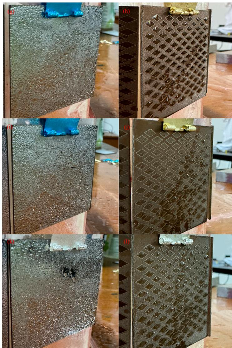
**Figure 35.** Comparison of untreated samples and superhydrophilic–superhydrophobic patterned samples in a 5 °C fog environment. Figure (a,b) is face I, figure (c,d) is face II, figure (e,f) is face III, figure (g,h) is face IV, figure (i,j) is face V, figure (k,l) is face VI.
