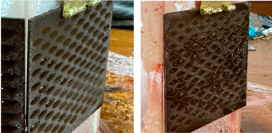
**Figure 28.** Side comparison of transverse diamond pattern and transverse ellipse pattern.
