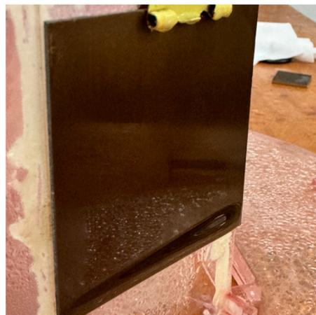
**Figure 5.** Water adhesion on the fully hydrophilic sample during the 20 min experiment.
