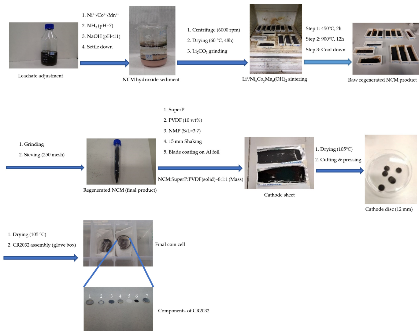
Figure 1. Flow of NCM regeneration and CR2032 coin cell assembly with coin cell components: 1: anode cap; 2: spring; 3: spacer; 4: Li block; 5: Celgard 2400 separator (Shenzhen, China) (wet with \text{LiPF}_6 ); 6: cathode disc; 7 cathode cap.
