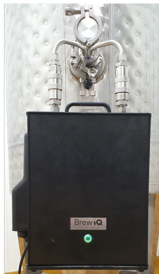
Figure 3. The Precision Fermentation BrewIQ fermentation monitor used for real-time monitoring of fermentation parameters.
