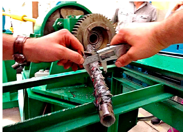
Figure 8. Exfoliation of the surface layer during rolling on the SVP-08 mill.
