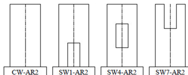
Figure 19. Wall specimens to study concrete compressive strength effect.
