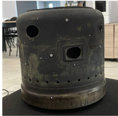
Figure 5. The combustion chamber body of the Capstone micro-GTU prepared for the 3D laser scanning process C 65 with reflective markings applied.
