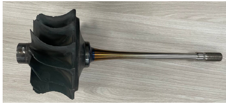
Figure 17. Detail of the rotor of the gas turbine of the Capstone C 65 micro-GTU installation.
