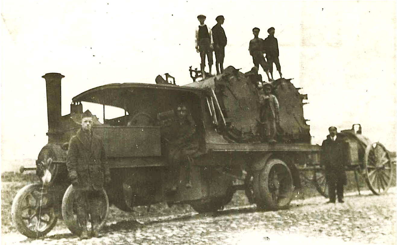
Figure 4. One of the 10 mobile Foden–Thresh Mobile Sterilizers sent to Poland by the APRE in 1919. The Foden lorry was steam powered and supplied steam to the Thresh disinfector [24,61].
