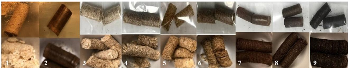
**Figure 8.** Illustrations of treated and non-treated pellets before (**top**) and after (**bottom**) moisture absorption test. From left to right: pellet made of raw sawdust (1), steam-treated (2), raw sawdust with 10% (3) and 20% ST (4), optimized torrefied sawdust with 10% (5) and 20% ST (6), torrefied sawdust at outside temperatures of 230 (7), 260 (8) and 290 °C (9) with 20% ST.
