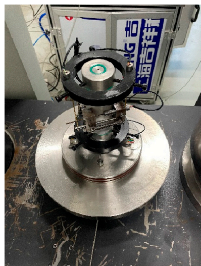
Figure 6. Coal sample installation process.
