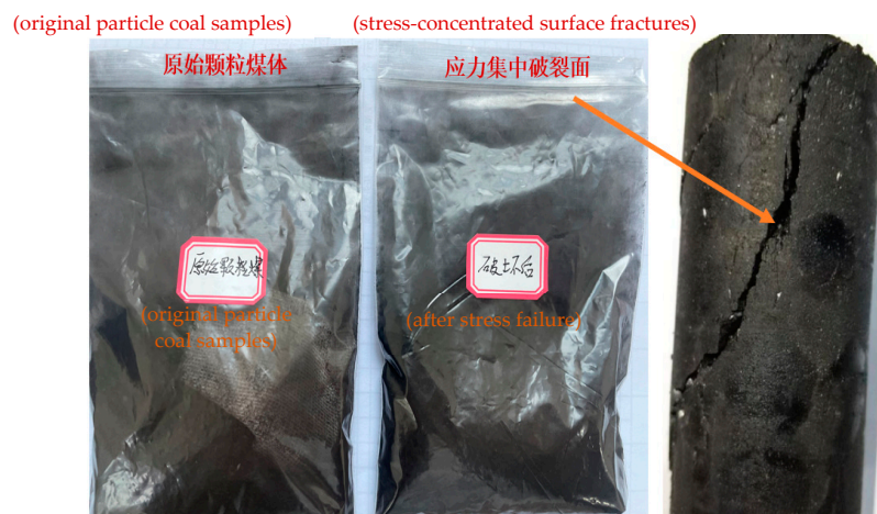
Figure 2. Sampling images and positions after stress load failure.
