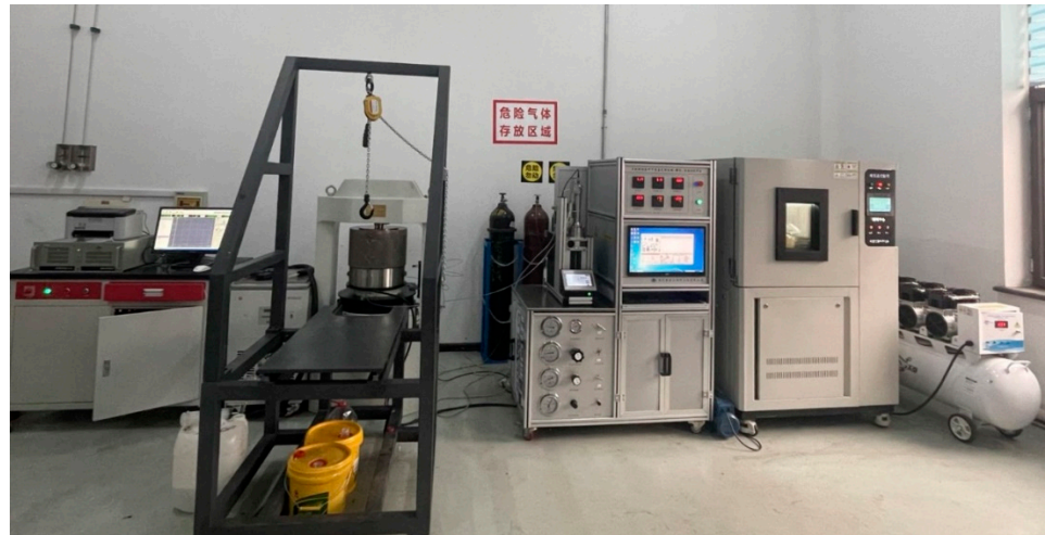
Figure 3. Experimental platform for gas adsorption of coal under stress load.
