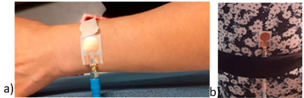
Figure 7. (a) Antenna located on the hand, (b) antenna located on the abdomen, both locations measured with and without the thin cloth between the antenna and the skin.
