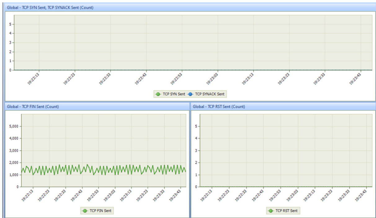
Figure 35. Number of different TCP packets sent during the TCP FIN attack for the video conversation.
