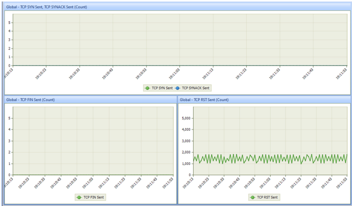
Figure 32. Number of different TCP packets sent during the TCP RST attack for the video conversation.
