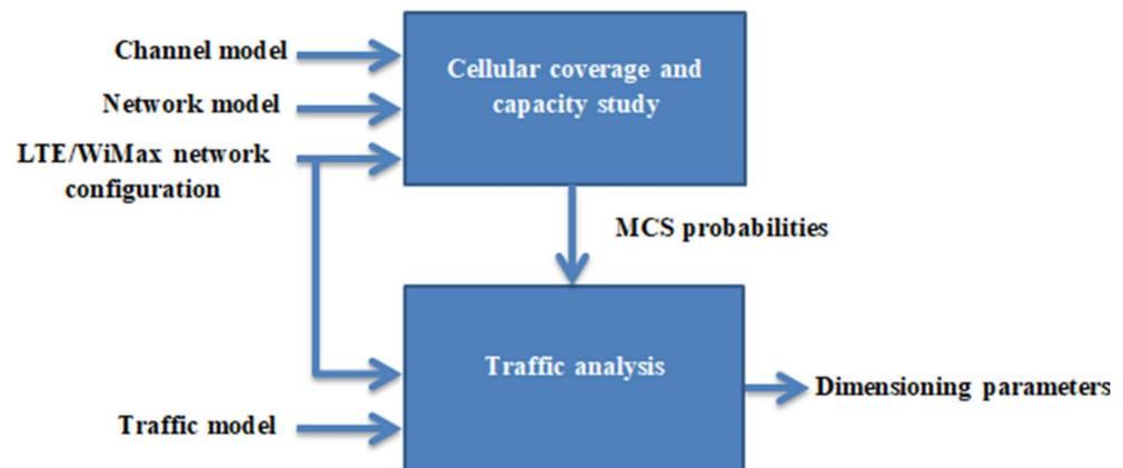
**Figure 2.** The system studied for the dimensioning study.
