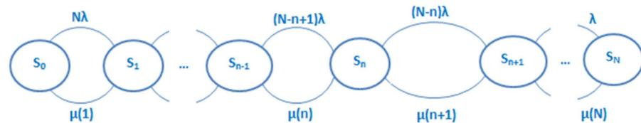
**Figure 1.** The Multidimensional Continuous-Time Markov Chain.
