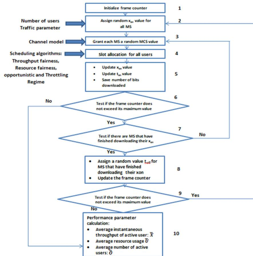
Figure 3. Simulator diagram.
