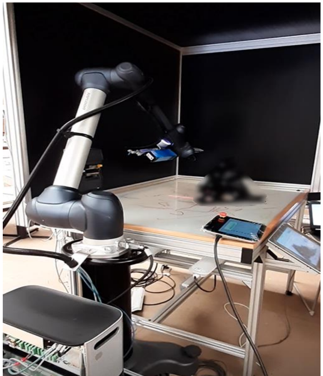
Figure 2. Industrial prototype for quality inspection.
