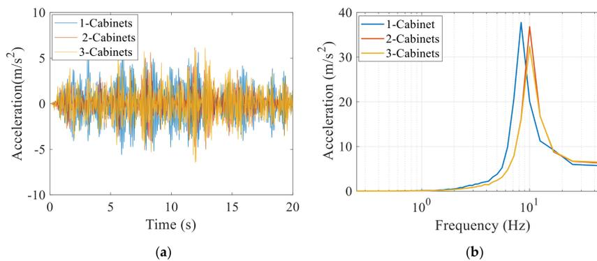
**Figure 13.** Cabinet response under the Artificial ground motion compatible with RG 1.60; (a) Acceleration response; (b) Maximum In-Cabinet response.
