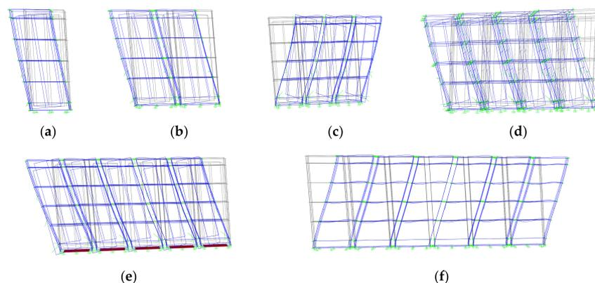
**Figure 10.** Numerical models for the grouping effect of the cabinets; (a) Single Cabinet; (b) Two cabinet assembly; (c) Three cabinet assembly; (d) Four cabinet assembly; (e) Five cabinet assembly; (f) Six cabinet assembly.
