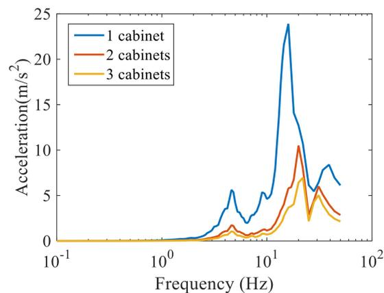
**Figure 19.** In-Cabinet response generated using empty cabinets (Salman et al., 2019).
