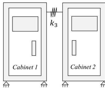
Figure 7. Typical assembly of two cabinets.
