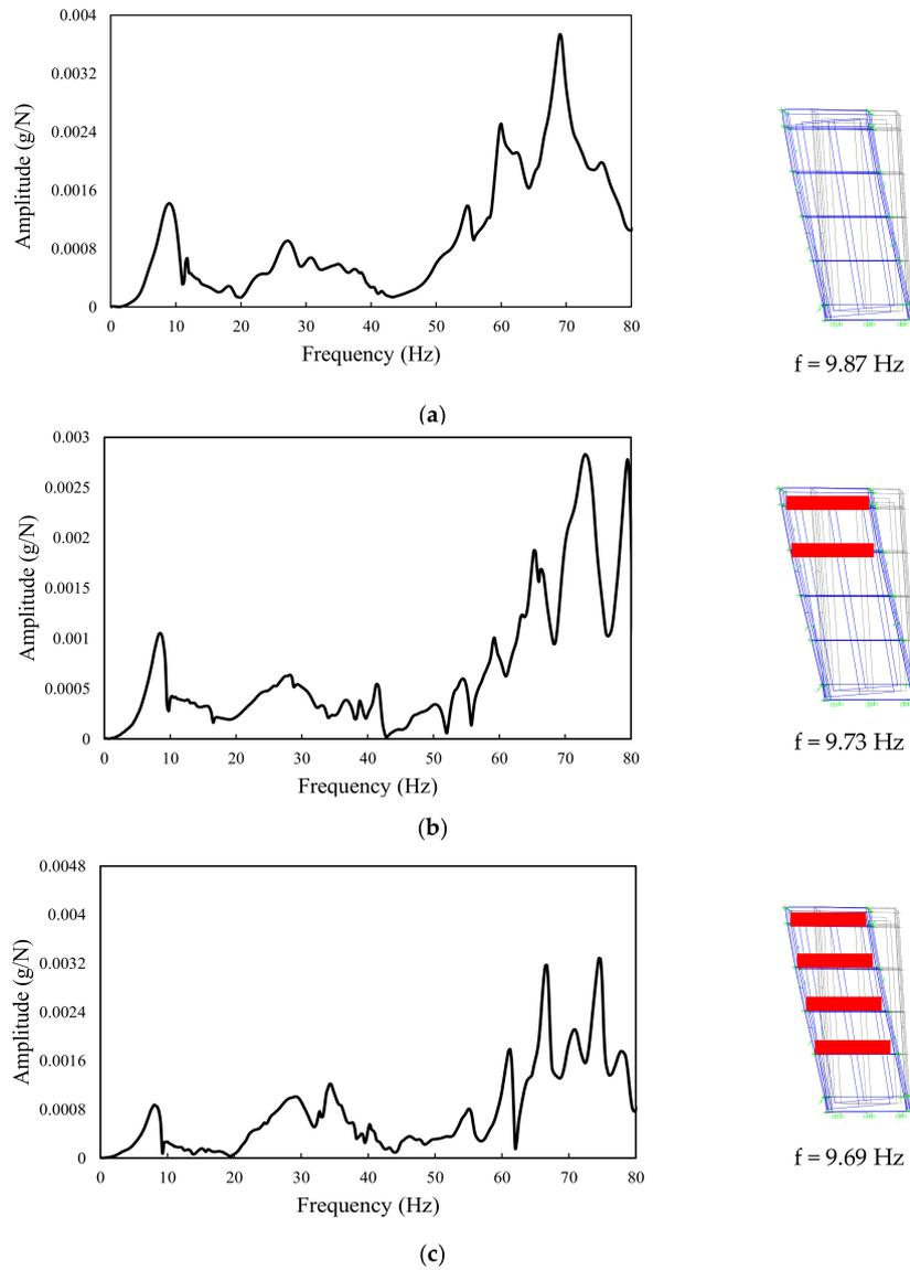
**Figure 6.** Natural frequencies from Experimental and Numerical modal analysis: (a) Empty Cabinet; (b) Loaded Cabinet at the top; (c) Fully loaded Cabinet.
