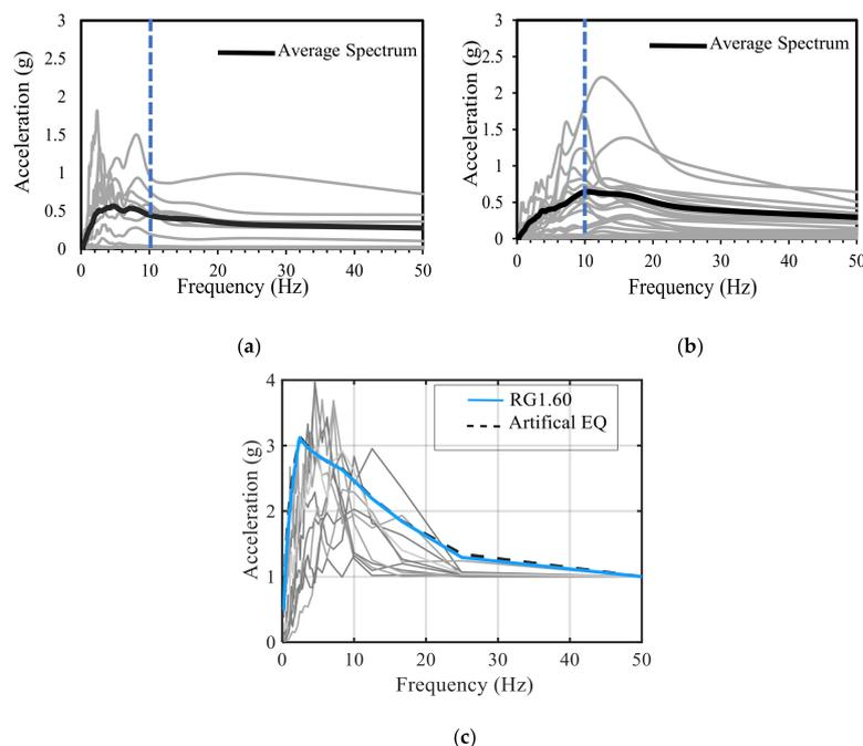
**Figure 11.** Seismic inputs for the ICRS generation: (a) Low frequency earthquakes (below 10 Hz); (b) High frequency earthquakes (above 10 Hz); (c) Scaled ground motions with artificial ground motions compatible with RG 1.60.
