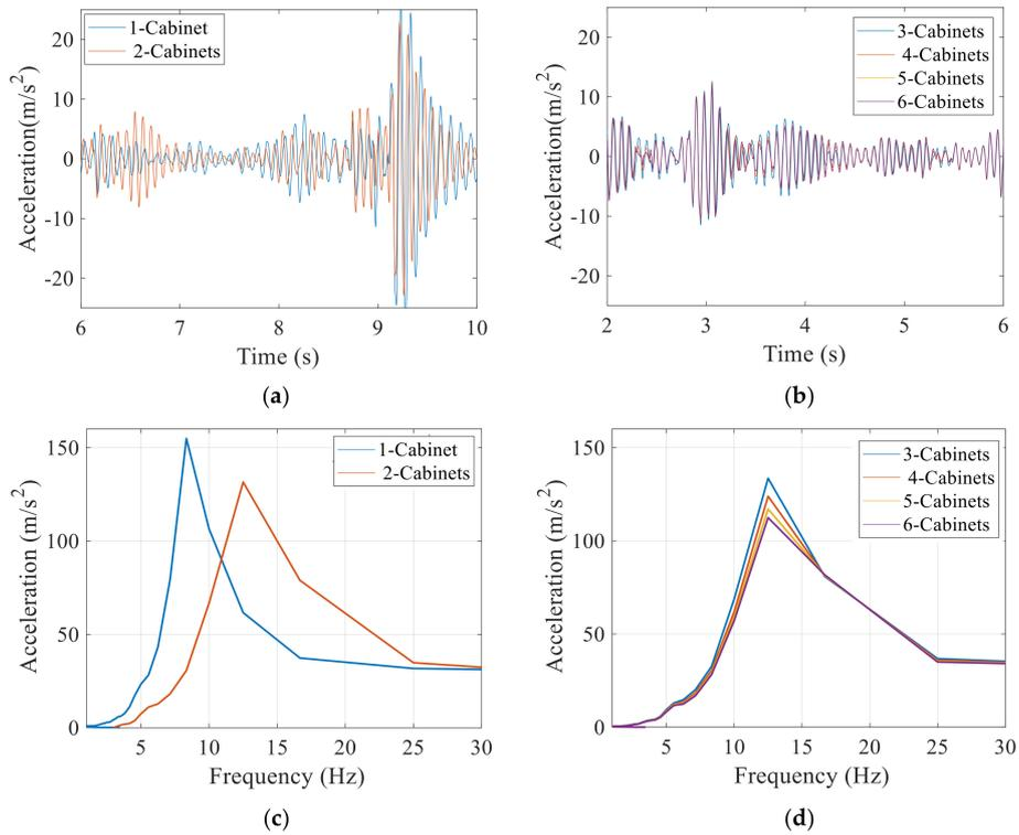
**Figure 16.** Seismic response of cabinets under Mexico Nahani Canada earthquake: (a) Acceleration response for one and two cabinets; (b) Acceleration response for multi-cabinets; (c) Maximum ICRS for one and two cabinets; (d) ICRS for multi-cabinets.
