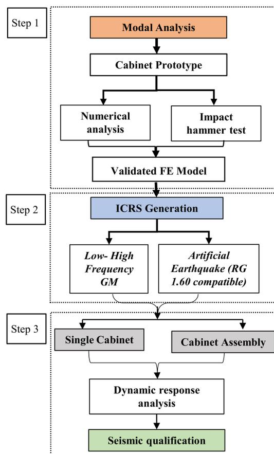
**Figure 1.** Schematic procedure for the seismic qualification of interconnected cabinets.
