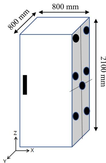
Figure 2. Installed accelerometers on the cabinet specimen.
