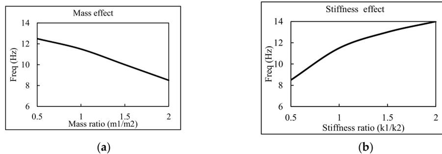
**Figure 9.** Effect on the natural frequencies of cabinets considering  $k_3$ ; (a) Effect of mass ratio; (b) Effect of stiffness ratio.
