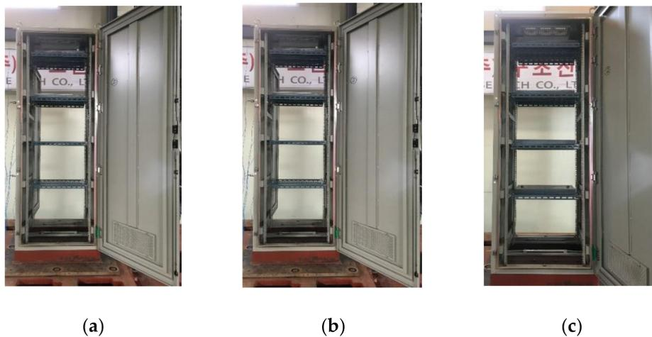
Figure 3. Cabinets prototype under different loading condition: (a) Empty cabinet; (b) Loaded at the top; (c) Fully loaded.
