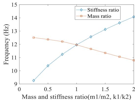
**Figure 12.** Variation in natural frequencies of two cabinets due to mass and stiffness ratio.
