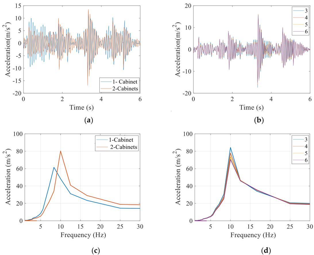
**Figure 14.** Seismic response of cabinets assemblies under Victoria\_ Mexico: (a) Acceleration response for one and two cabinets; (b) Multi-cabinets acceleration response; (c) Maximum ICRS for one and two cabinets; (d) Maximum ICRS for multi-cabinets.
