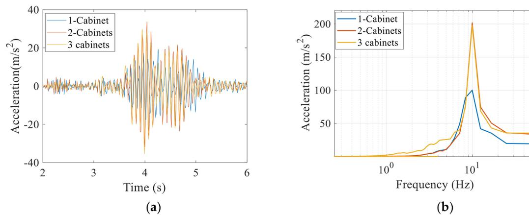
**Figure 15.** Seismic response of cabinets under the Goungju Earthquake: (a) Acceleration response; (b) Maximum In-cabinet response spectra.
