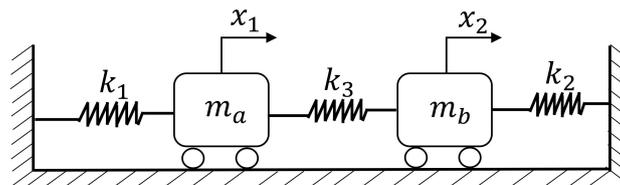
Figure 8. Mass-spring model of two interconnected cabinets.
