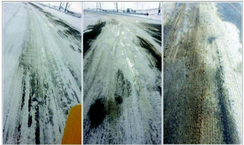
Figure 7. Sand applied on icy road surface at the IRRF test road in Canada [58].
