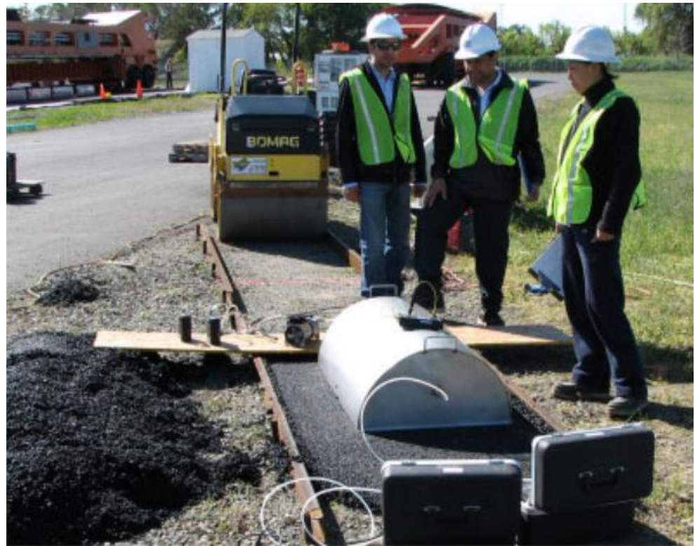
Figure 8. Measuring VOCs using the transportable flux chamber [67].
