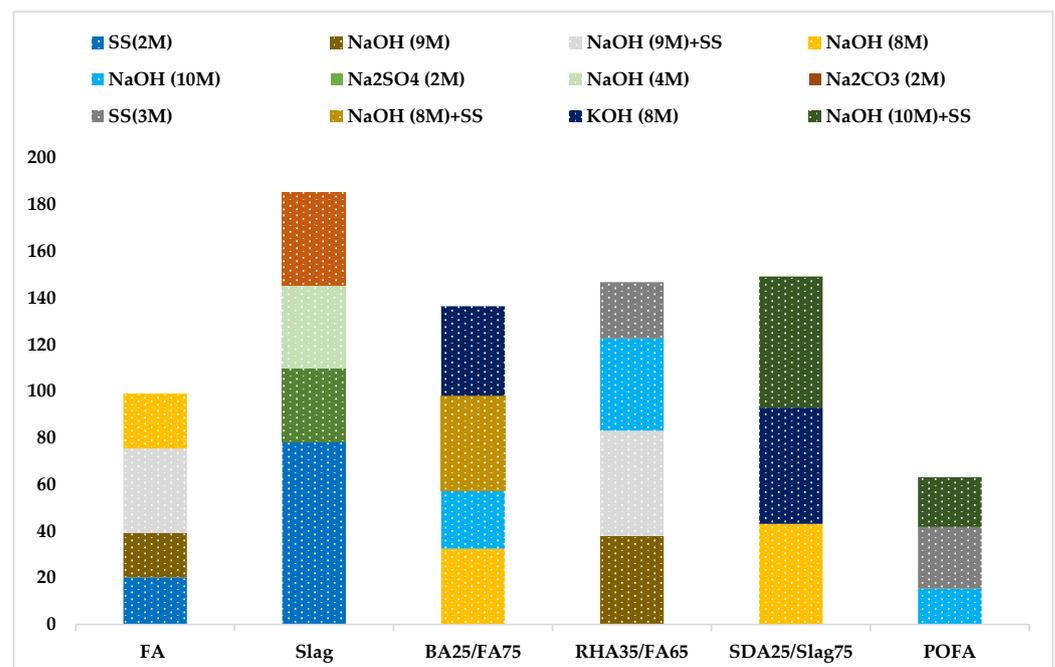
Figure 10. Impacts of AA on compressive strength of AAB in 28 days.
