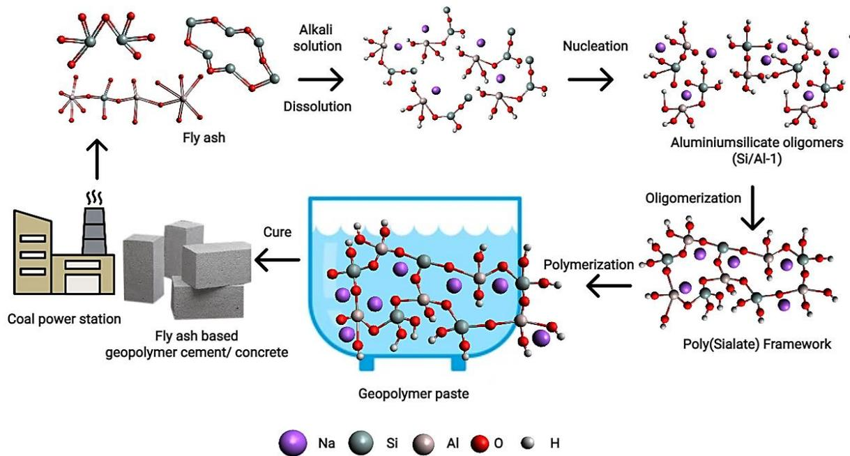
Figure 3. Geo polymerization process of fly ash (FA).
