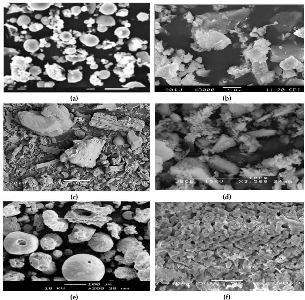
**Figure 9.** Residual ashes' SEM micrographs. (a) FA [113], (b) GGBFS [113], (c) SBA [93], (d) RH-SiO<sub>2</sub>, (e) POA [97] and (f) SA [116].
