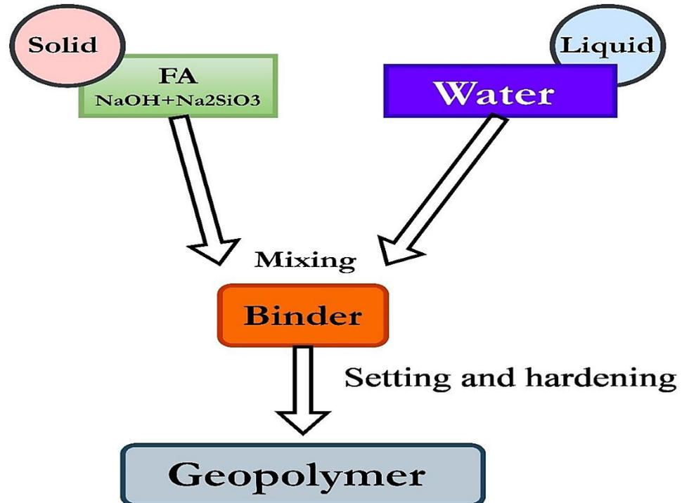
Figure 4. Dry mixing geo polymerization.
