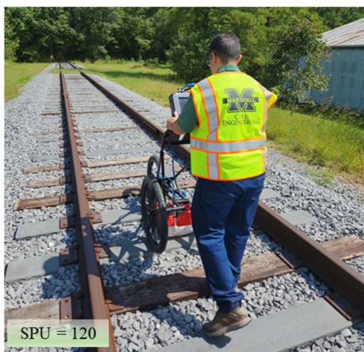
GPR push-cart system (ERDC test facility)
