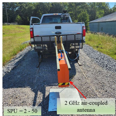
GPR hi-rail system (ERDC test facility)
