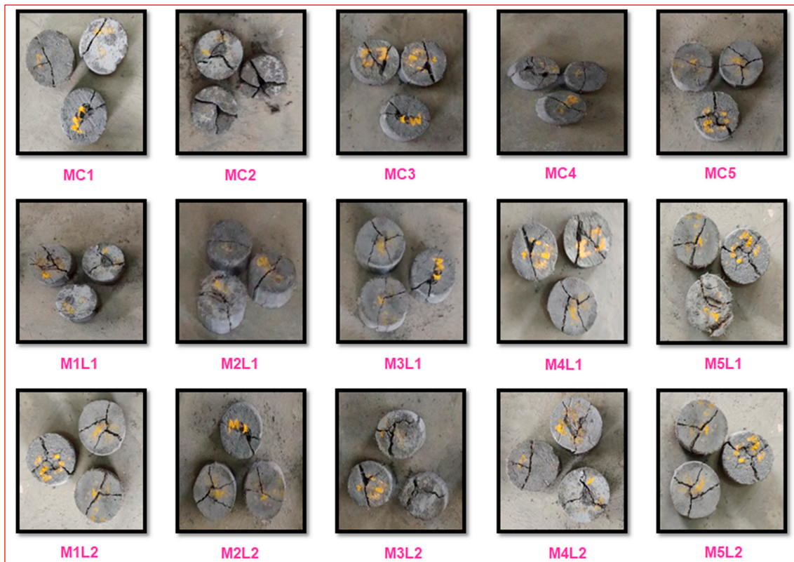
Figure 11. Typical failure patterns of disc specimens of QBC.
