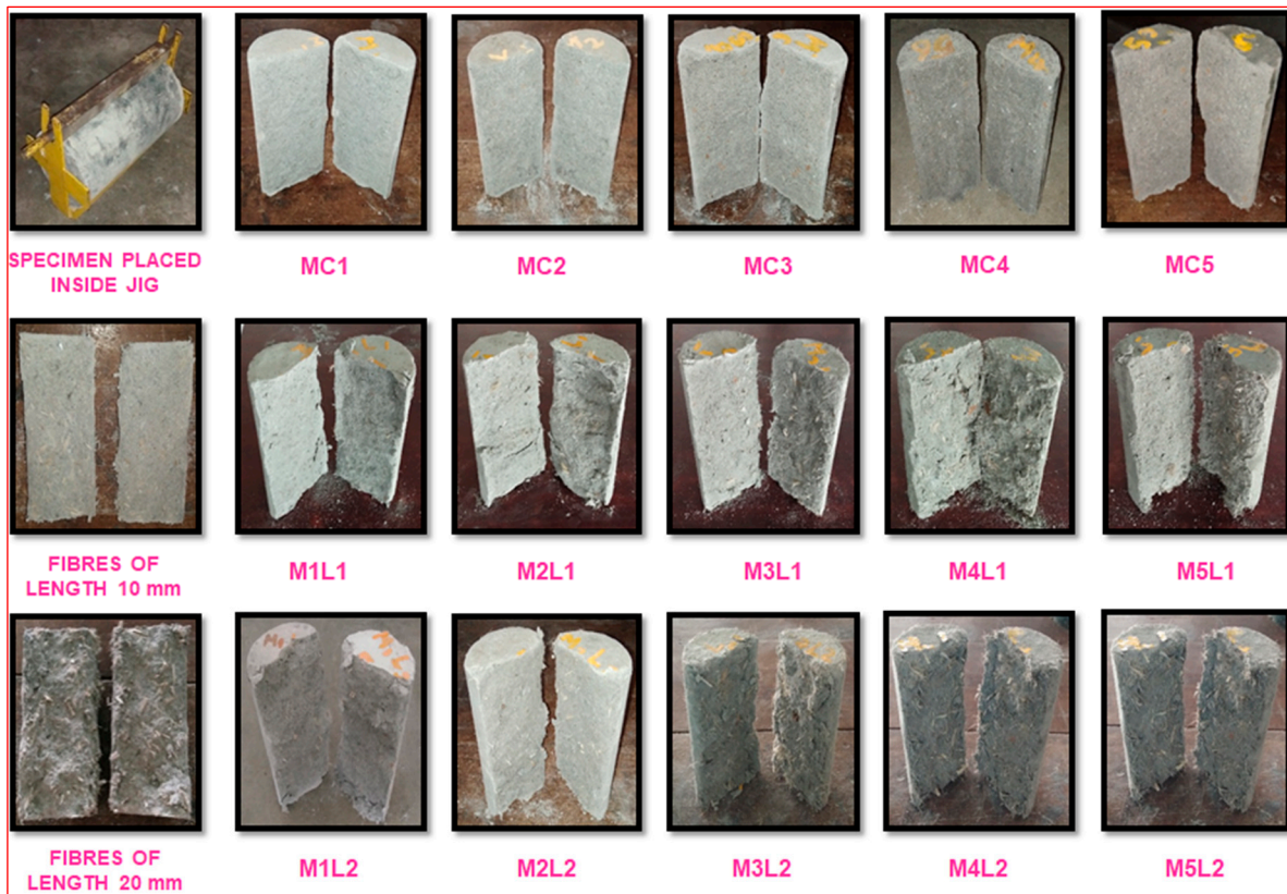
Figure 9. Typical failure patterns of cylinder specimens of QBC.
