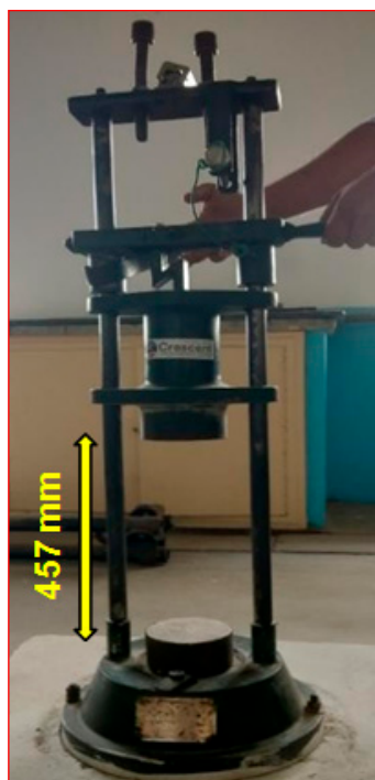
Figure 4. Impact strength test set-up.
