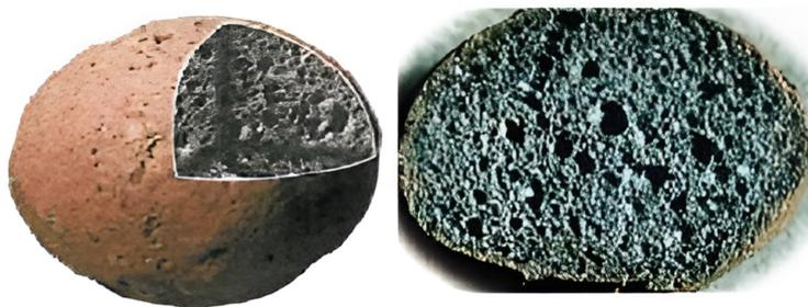
**Figure 12.** Air-filled cavities and interconnected holes of different sizes in LECA [104].
