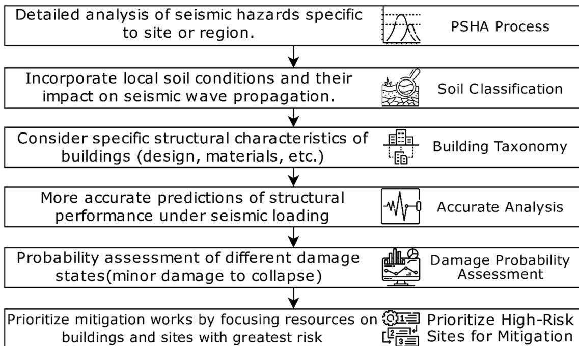
**Figure 3.** Process and application of developing building- and site-specific fragility curves.
