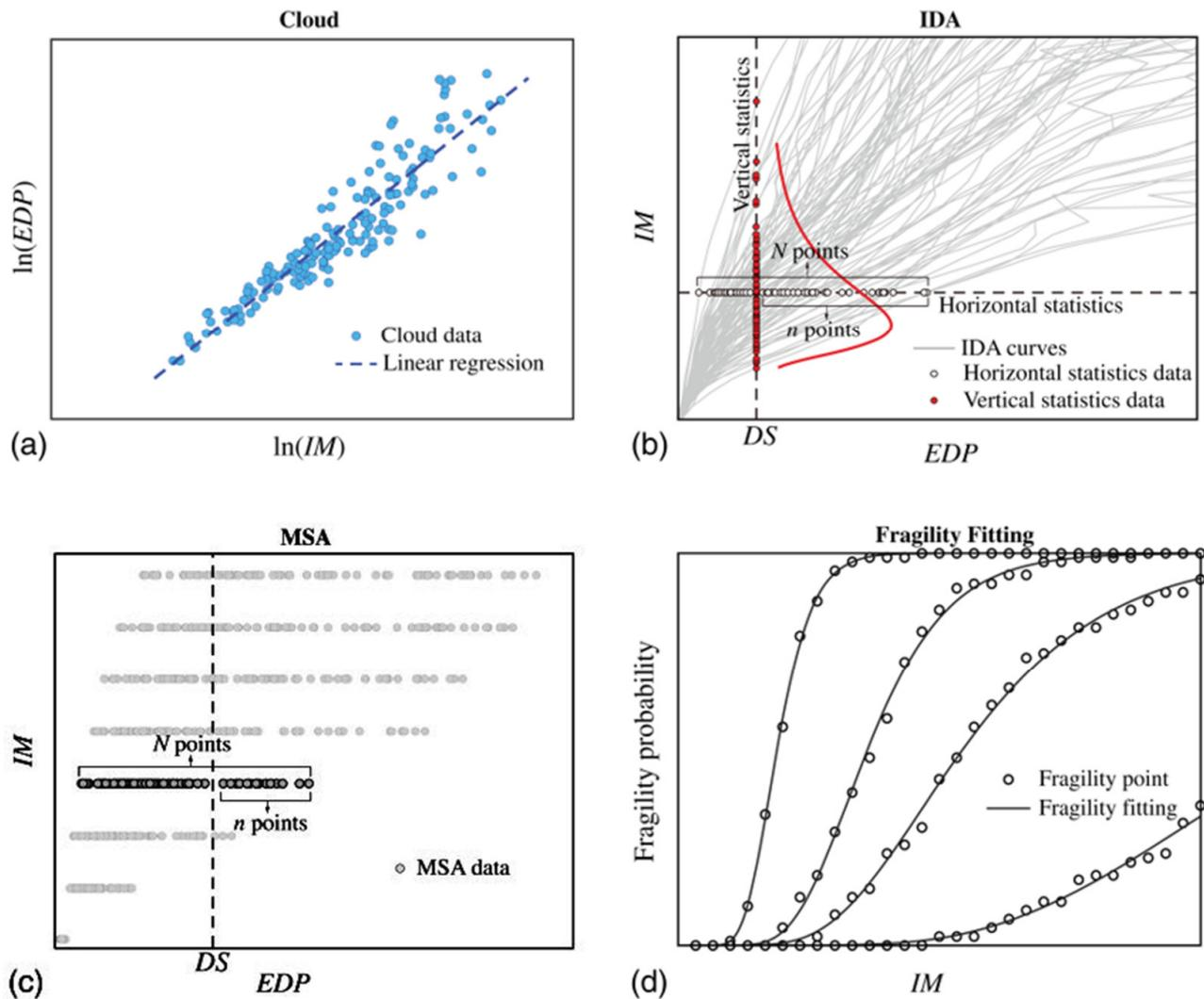
**Figure 5.** Pang and Wang [50] illustration of fragility modeling: (a) using logarithmic linear regression to relate intensity measure (IM) to engineering demand parameters (EDPs) in Cloud; (b) employing IDA curves to estimate damage probabilities in two distinct approaches; (c) utilizing MSA data to forecast damage probabilities; and (d) developing fragility curves based on fitting methods in both IDA and MSA. (Reprinted with permission from Ref. [50], 2021, ASCE).
