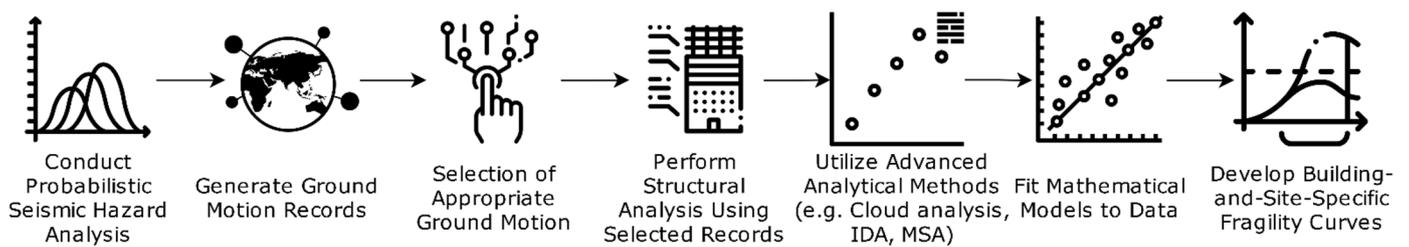
**Figure 4.** Process of creating highly accurate and relevant seismic fragility curves for diverse structural types through PSHA-based record selection.
