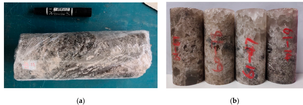
Figure 1. Core pillar and standard rock sample for experiment (a) for core pillar, (b) for standard core.
