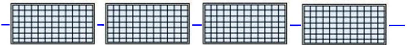
Figure 4. Solar voltaic panels in a series configuration [9].
