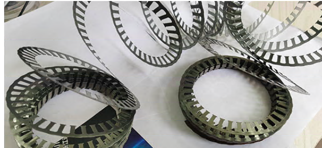
Figure 11. Spiral core assembly [73].
