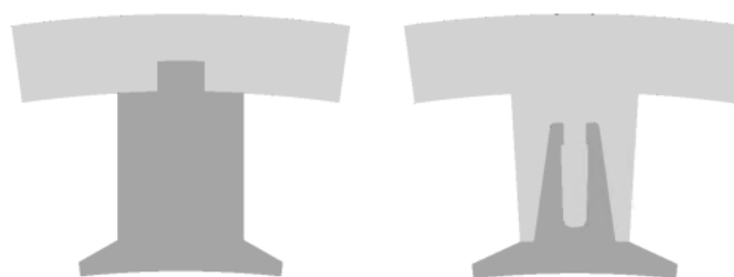
Figure 9. Interlocking shapes used for radially segmented stator tooth and back iron structures [29].
