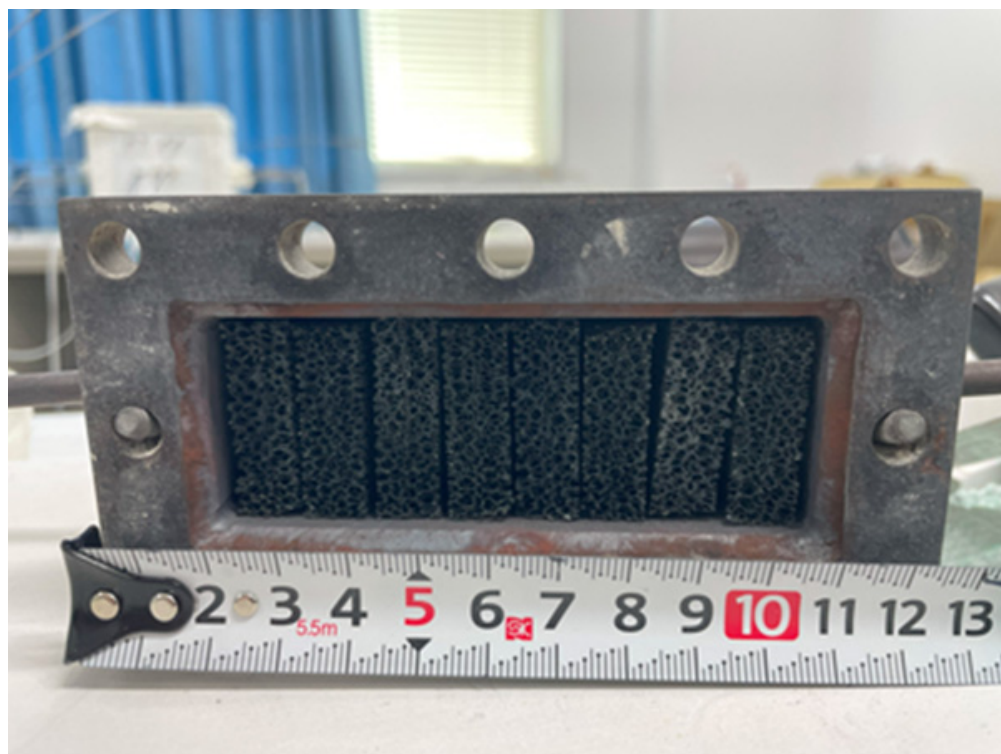
Figure 3. Photograph of the charged Ni/Cr/Ru catalyst in the reactor.
