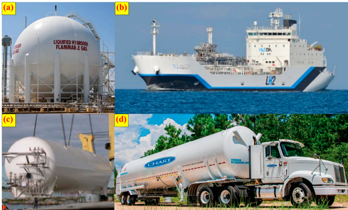
Figure 1. Typical methods for the storage and delivery of liquid hydrogen: (a). Spherical tank (NASA, Washington, D.C., Washington, United States, 3200 m 3 ) [8]; (b). Liquefied hydrogen carrier ship (Kawasaki, Tokyo, Japan, 1250 m 3 ) [9]; (c). Cylindrical horizontal tank (Linde, Pullach, Germany, 300 m 3 ) [10]; (d). Transport trailer (Chart, Rancho Dominguez, CA, United States, 66.7 m 3 ) [11].
