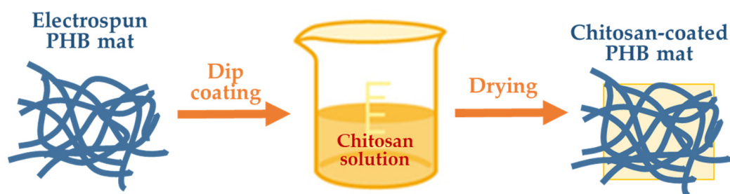
Scheme 1. Schematic representation of the preparation of chitosan-coated PHB mats.
