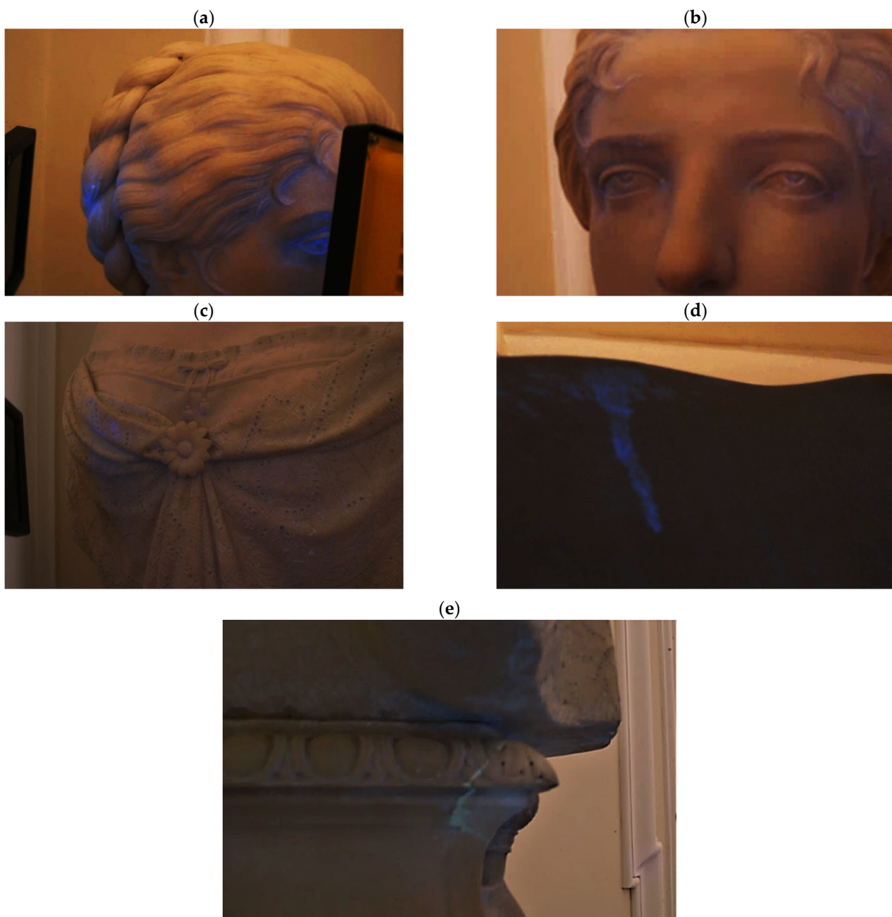
Figure 4. Details of visible induced fluorescence areas under UV light. (a) Head: Hair and eye. UV fluorescence of calcite polymorphs; (b) Head: face area. UV fluorescence of calcite polymorphs; (c) Body: drippings. UV fluorescence; (d) Back: drippings. UV fluorescence; (e) Base: adhesive UV fluorescence.
