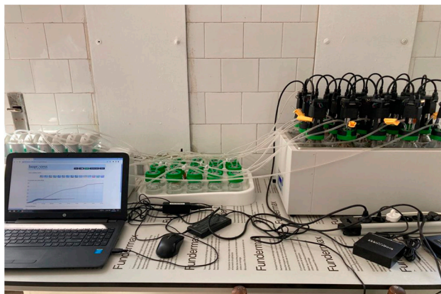
Figure 1. Automatic gas flow measuring system used for anaerobic digestion.
